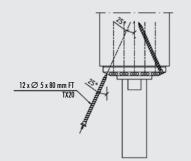
After centring the head plate, screw in the 12 full-thread 5.0 x 80 mm screws at an angle of 25° without pilotdrilling.
