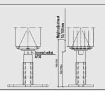
The protective sleeve and the baseplate can be reinstalled after all screws are fitted. After the post is erected with the post foot installed, it can be anchored on a concrete foundation with two or four cavity-wall ties or concrete bolts. Once the foot is installed on the socket, its height can be adjusted using an AF30 spanner.
