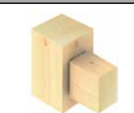
Secondary beam - support
