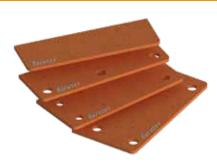
The Eurotec SonoTec Angular Decoupler forms the perfect complement to the Eurotec Shearing Angles and the CLT System Angle. The underlay is made from SK04, which is a compound formed from cork and natural rubber. The product is suitable for vibration damping applications in which very high insulation values are required. SonoTec angular decouplers are used as invisible insulators (pads/strips) with a low resonance frequency and a medium-low load.
