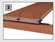
Align and fix the next board, screw down with the T-Stick until all boards are fastened.
