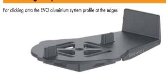
To prevent individual stone slabs from slipping, the stone edge clips are to be screwed to the aluminium substructure in the edge area. The clips have a screw channel in the middle for this purpose.
