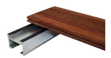
b) If WPC boards are used, the centre distance e between the profiles must not exceed 400 mm!
