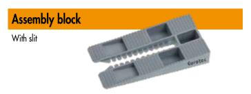
Load-bearing **Dimensions** Height adjustment Colour PU Art. no. [mm]<sup>a)</sup> capacity [kg] [mm] 964550 10 x 70 x 35 ≤ 200 10 - 15 Yellow 1000 10 x 77 x 38 10 - 15 964551 ≤ 200 White 1000 15 - 22 964552 15 x 88 x 43 ≤ 300 Grey 500 964553 25 x 140 x 43 ≤ 500 25 - 42 364 a) Height x length x width
