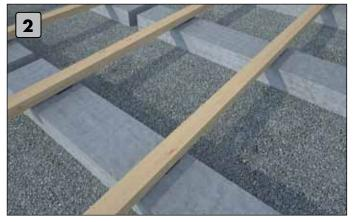
Concrete elements are laid in a gravel bed.
