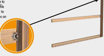
The remaining Façadeclips Rhombus can be mounted along the profile. Place the clips between the board and the substructure joist and fix them with the enclosed screw. The screws of all clips must be sufficiently tightened. The information provided as in the remark applies to fixed points in the event of horizontal installation.
