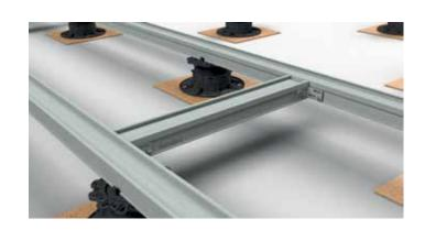
b) e.g.: spacing between profiles = 550 mm; payload = 2,0 kN/ $m^2$   $\rightarrow$  max. span of the profile = 650 mm. d Payloads according to DIN EN 1991-1; roof terraces = 4 kN/ $m^2$ , patios for public use = 5 kN/ $m^2$ .
