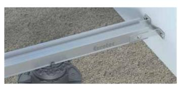
The **EVO wall-connection bracket** is ideal for use as a position anchor for deck substructures made of aluminium. The bracket is used to fasten the EVO aluminium system profile directly to the wall. Two EVO wall-connection brackets are needed per aluminium profile. The slots in the wall-connection bracket allow the substructure to expand without problems and therefore prevent it from shifting out of position.
