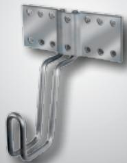
With the Topduo double-threaded screw, the additional point loads arising due to a photovoltaic or solar-thermal system are safely transferred to the rafter. The roof hooks are fastened to the rafter by means of two screws that pass through the entire assembly height of the over-rafter insulation.
